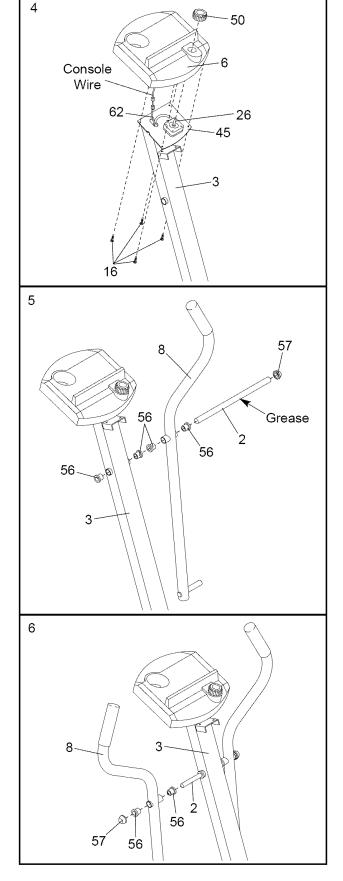
6. Slide the other Handlebar (8) onto the Pivot Axle (2). Secure the Handlebars to the Upright (3) by tapping a 5/8" Axle Cap (57) onto the end of the Pivot Axle. 7. Attach the T-handle (10) to the Upright (3) with two M6 x 16mm Button Screws (54) and two M6 Nylon Locknuts (55).
